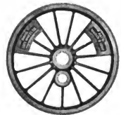
Fig. 1326. Cast-Steel Driving Wheel Center with Davis Counterbalance. Davis Loco. Wheel Co.
